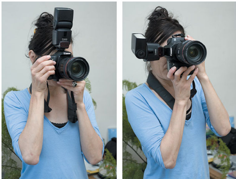
FIGURE 9.10 If your flash can tilt and swivel, it's easy to keep it pointed at the ceiling as you change from portrait to landscape orientation.
